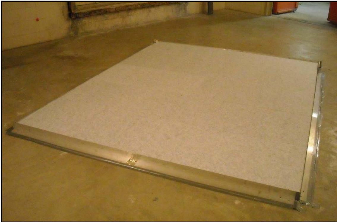
**Figure 2 – Specimen Prepared For Sound Absorption Testing**
